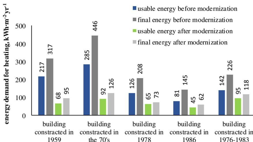
Fig. 1. Energy demand for heating per unit area
