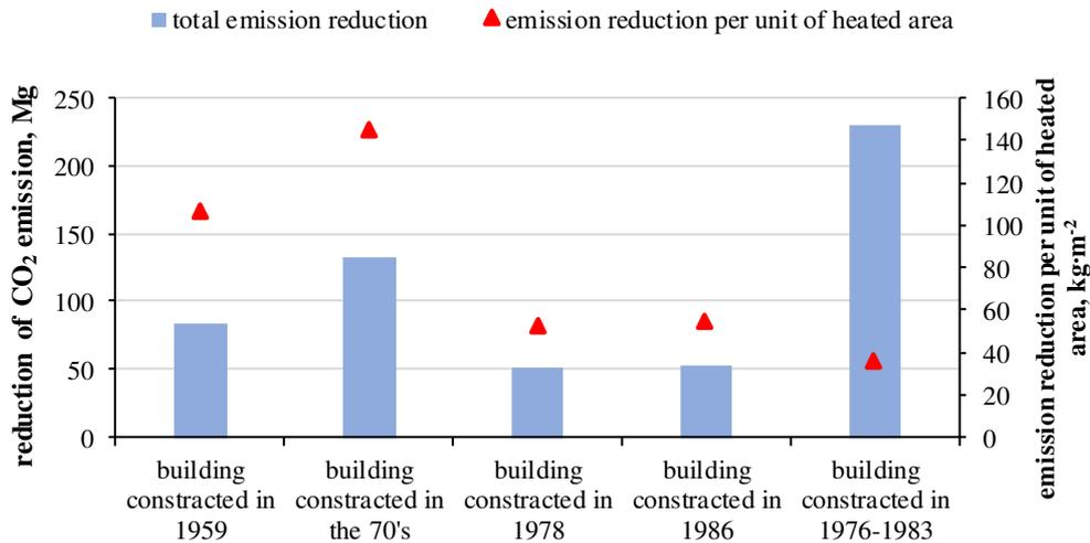
Fig. 3. Total reduction of CO<sub>2</sub> emission and reduction per unit of heated area
