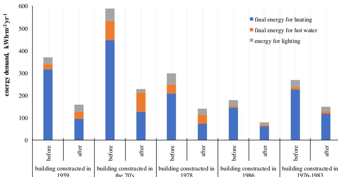
Fig. 2. Structure of energy consumption in analysed buildings before and after deep thermal modernization
