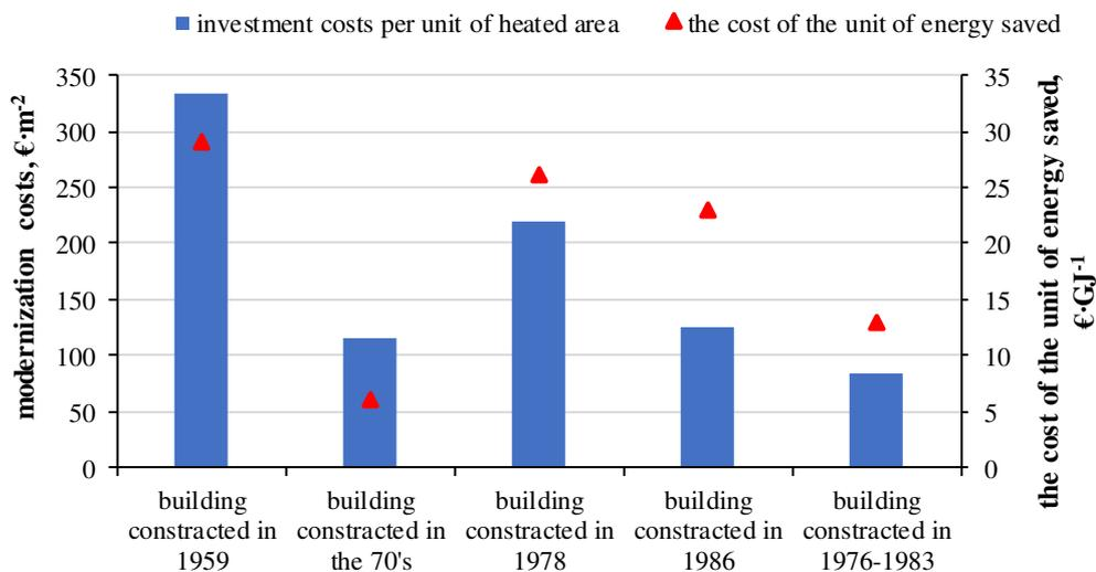
Fig. 4. Investment costs per unit of heated area and cost of unit of energy saved
